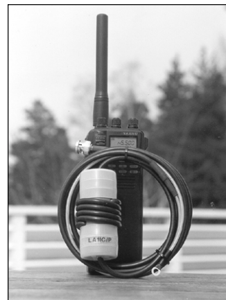
Rolled-up and ready to go, the 2m version of the feedline vertical.
